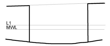
The two watertight bulkheads specified above may be replaced by a watertight cockpit. In this case the cockpit sole shall be above L1 level and the cockpit shall have at least two self-bailers. Openings for control lines shall meet the above requirements and any hatches shall maintain the watertight integrity of the cockpit. The weight of each bulkhead, including the weight of the adjacent ring frame if fitted, shall be not less than 6.5kg.
